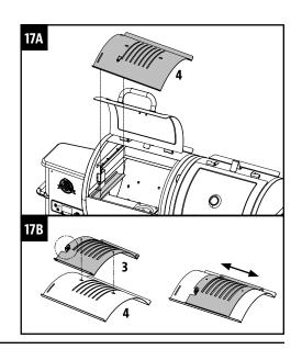
the left side, and the two slots on the Flame Broiler Main Plate will fit into the rounded ledge above the burn pot. It will sit slightly at a downward angle. Note illustration 17A.
